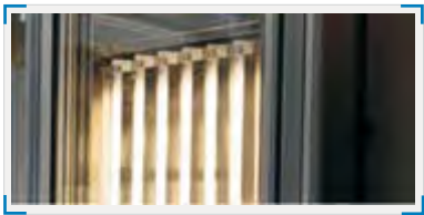
FIT D - Climatic chambers with lamps installed in the door
