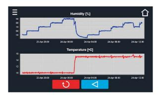
To enlarge a fragment of the graph press anywhere on the graph and swipe both right and down at the same time to. By swiping left you can return to the normal size of the graph.
