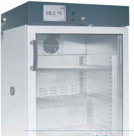
Cooled incubators (ST) can provide a stable temperature between +3...+70°C regardless of ambient conditions.
